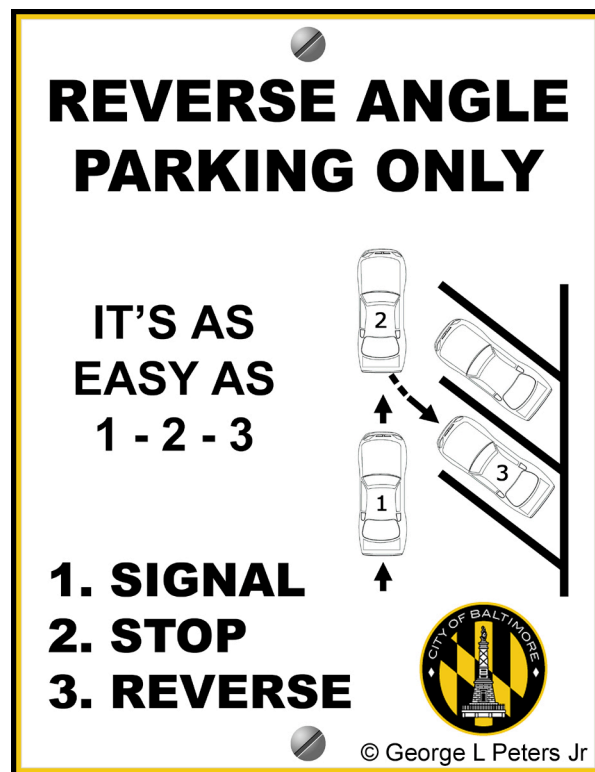
This is a rendering of what a posted Reverse angle parking sign may look like
